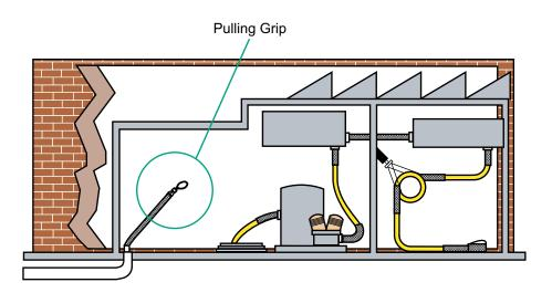
CAUTION: Never use grip to approximate breaking strength. Refer to technical data page for safety and working load factors. Banding is necessary to guard against accidental release of grip and provide maximum reliability.
