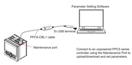
When using the maintenance port, power is provided from the USB port. Do not supply power to the controller through the terminals until disconnected from the maintenance port.
