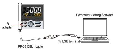
Connect to a powered PPC5 series controller using the IR adapter to upload/download and set parameters, monitor operations, tune control loops, and file management.
