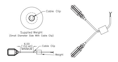
Float Travel is proportional to distance between float body and weight or anchor point.
