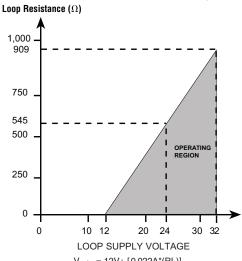
V<sub>min</sub> = 12V+ [0.022A\*(RL)] (Includes a 10% safety factor)
