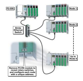
Add up to 8 Remote Bases using P2-RS Slave modules and up to 16 GS Drives on the Remote I/O Ethernet Network
