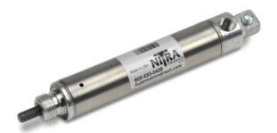
NITRA pneumatic stainless steel round body, interchangeable, non-repairable cylinder, 7/8 inch bore, 1/8 NPT port, single acting, spring return, rear pivot mount (pivot pin included).
