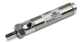
NITRA pneumatic stainless steel round body, interchangeable, non-repairable cylinder, 7/8 inch bore, 1/8 NPT ports, double acting, front nose mount.
