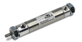
NITRA pneumatic stainless steel round body, interchangeable, non-repairable cylinder, 7/8 inch bore, 1/8 NPT ports, double acting, double end mount.
