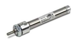
NITRA pneumatic stainless steel round body, interchangeable, non-repairable cylinder, 7/16 inch bore, #10-32 ports, double acting, front nose mount.
