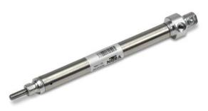
NITRA pneumatic stainless steel round body, interchangeable, non-repairable cylinder, 7/16 inch bore, #10-32 port, single acting, spring return, rear pivot mount (pivot pin included).
