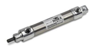
NITRA pneumatic stainless steel round body, interchangeable, non-repairable cylinder, 3/4 inch bore, 1/8 NPT ports, double acting, rear pivot mount (pivot pin included).
