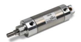
NITRA pneumatic stainless steel round body, interchangeable, non-repairable cylinder, 2 inch bore, 1/4 NPT ports, double acting, double end
