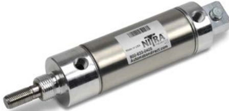
Cylinder, 1-1/2 in bore, double acting, rear pivot mount, magnetic piston
