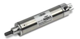
NITRA pneumatic stainless steel round body, interchangeable, non-repairable cylinder, 1-1/16 inch bore, 1/8 NPT port, single acting, spring return, rear pivot mount (pivot pin included).
