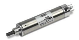
NITRA pneumatic stainless steel round body, interchangeable, non-repairable cylinder, 1-1/16 inch bore, 1/8 NPT port, single acting, spring return, rear pivot mount (pivot pin included).
