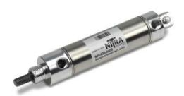
NITRA pneumatic stainless steel round body, interchangeable, 1-1/16 inch bore, 1/8 NPT ports, double acting, rear pivot mount (pivot pin included).
