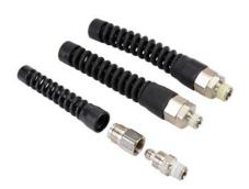
NITRA™ air or water threaded fittings with strain relief are excellent for use on our Hybrid PVC polyester reinforced hose. They are comprised of a nickel-plated brass body and threads with an impact resistant acetal strain relief. Threaded sealant is pre-applied.
