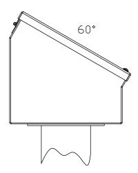
CONSOLET CAN BE POSITIONED AT 30° OR 60° ANGLE
