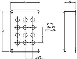
PBXD HOLE ARRANGEMENTS 0 0 0 000 $\bigcirc$ 0 0 0 0000 000 0 00 0 00  $\bigcirc$ 000  $\circ$  $\bigcirc$  $\circ$  $\bigcirc$ 000PBXD1 **PBXD2** PBXD3 PBXD4 PBXD4S PBXD6 PBXD9 PBXD10 PBXD12 0  $\bigcirc$ 0 0.67 -[17.0] 0.19 0 0 [4.8] 0000 00000 00 00000 000  $\circ$ 0 0000 ø1.20 -[ø30.5] 0000 00000 00 0000 0000 0 000 00000 STANDARD 4-WAY
