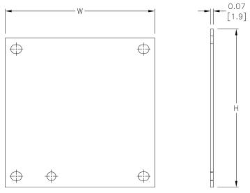
Note: Perforated panels have 0.13in [3 mm] diameter holes at 0.25in [6 mm] spacing.
