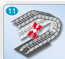
Installation option: Horizontal/vertical, combined
