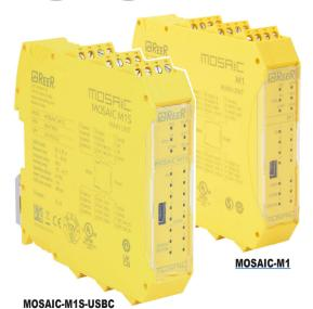
MOSAIC M1, M1S, or M1S-USBC controller units are able to interface with up to 14 individual expansion modules (up to a maximum of 4 of any one module type).
