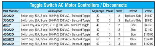
\*Motor controller only ("Not suitable as disconnect")
