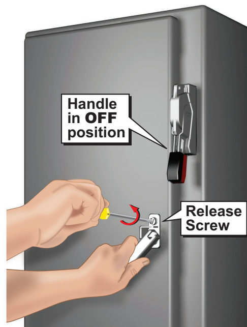
Safety Handle shown on enclosure
