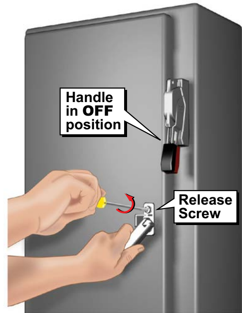
Safety Handle shown on enclosure
