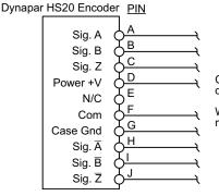
Connections to equipment determined by customer.
