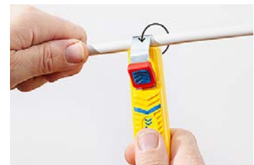
Adjustable dial for blade height
