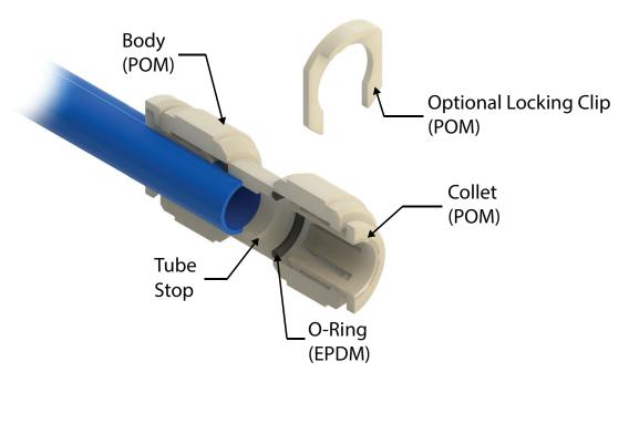
Push-to-Connect Fitting Cut-away Diagram
