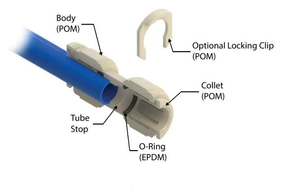
Push-to-Connect Fitting Cut-away Diagram
