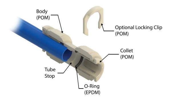
Push-to-Connect Fitting Cut-away Diagram
