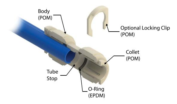
Push-to-Connect Fitting Cut-away Diagram
