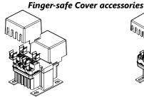
Sample Assembly Drawing for Finger Guard Installation (for 50, 75 and 100VA)
