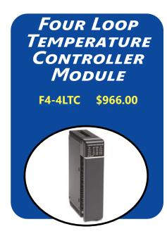
The temperature is read directly into the F4-4LTC with the on-board RTD or thermocouple inputs. If the temperature is not at the target value (setpoint), then the control outputs are automatically activated. The F4-4LTC also provides automatic tuning of the control loops, so the module can easily adapt to changing temperature and process conditions. And since the F4-LTC is an intelligent DL405 module, you can easily use simple ladder logic in a DL405 CPU for ramp and soak setpoint changes.
