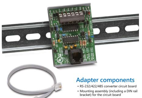
• 1 ft. modular cable with two RJ12 6P6C plugs
