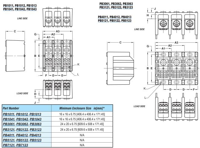
\*Note: Terminal block SCCR determined based on testing in minimum-size enclosure
