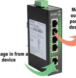
Message is sent out only from the port connected to destination device
