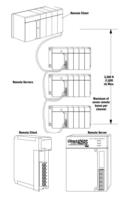
You can assign normal input and output addresses to the remote points, or you can assign special remote I/O addresses. The Remote Client sends the remote I/O information to the CPU. The communication between the Remote Client and the CPU is asynchronous to
