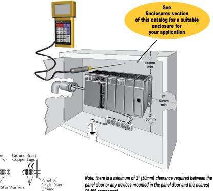
panel door or any devices mounted in the panel door and the nearest DL405 component.
