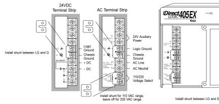
Recommended screw torque: 10.6 lb-in (1.2 Nm)
