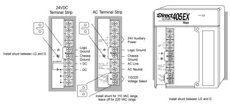
Recommended screw torque: 10.6 lb-in (1.2 Nm)
