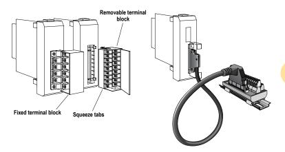
Z/PLinks eliminate the tedious process of wiring PLC I/O terminal blocks.
