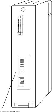
DIP Switches for communications and Protocol Setup
