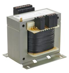
BLOCK control transformer, open core, 800 VA, 1-phase, 208-600 VAC selectable, 115/230 VAC secondary, 50/60 Hz, panel mount.
