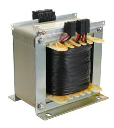
BLOCK control transformer, open core, 3.2 kVA, 1-phase, 208-600 VAC selectable, 115/230 VAC secondary, 50/60 Hz, panel mount.
