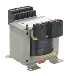
BLOCK control transformer, open core, 250 VA, 1-phase, 208-600 VAC selectable, 12/24 VAC secondary, 50/60 Hz, panel or 35mm DIN rail mount.
