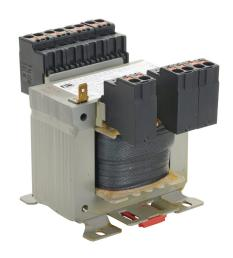
BLOCK control transformer, open core, 100 VA, 1-phase, 208-600 VAC selectable, 12/24 VAC secondary, 50/60 Hz, panel or 35mm DIN rail mount.
