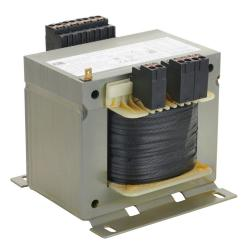
BLOCK control transformer, open core, 1 kVA, 1-phase, 208-600 VAC selectable, 115/230 VAC secondary, 50/60 Hz, panel mount.
