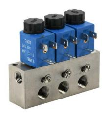
CFA solenoid valve bank, (3) stations, 2-port (2-way), N.C., 1/4in female NPT inlet(s), 1/4in female NPT outlet(s), Cv=0.14, individual metering, stainless steel body, 24 VDC, 4W, 11mm DIN style wiring plug.
