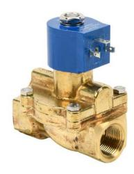
GC Valves solenoid valve, 2-port (2-way), 2-position, N.C., brass body, Viton seal(s), 3/4in female NPT inlet(s), 3/4in female NPT outlet(s), Cv=6.1, 1 psi minimum operating pressure, 120 VAC operating voltage, 18mm DIN style wiring plug.
