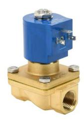
GC Valves solenoid valve, 2-port (2-way), 2-position, N.C., brass body, Viton seal(s), 1/2in female NPT inlet(s), 1/2in female NPT outlet(s), Cv=4.3, 0 psi minimum operating pressure, 120 VAC operating voltage, 18mm DIN style wiring plug.
