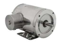
IronHorse MTS premium efficiency AC induction motor, washdown, inverter rated and hazardous location, 3/4hp, 3-phase, 208-230/460 VAC, 3600rpm, TENV, 56C frame, 304 stainless steel, C-face/rigid base mount.
