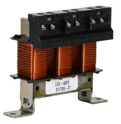
AutomationDirect LR2 series line reactor, 480 VAC, 1/2hp, 3-phase, 1.1A, 3% impedance, input or output side. For use with multiple AC drives.
