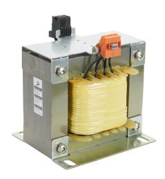
BLOCK control transformer, open core, 2 kVA, 1-phase, 240/480 VAC, 120 VAC secondary, 50/60 Hz, panel mount.
