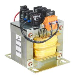
BLOCK control transformer, open core, 500 VA, 1-phase, 240/480 VAC, 120 VAC secondary, 50/60 Hz, fused, panel mount.
